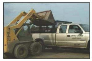
Turn your pick-up into a dump truck with our 6' or 8' dump insert. Complete with a 4" double acting hoist, this dump insert can handle over 2 tons of payload. Perfect for mulch, stone and firewood.
